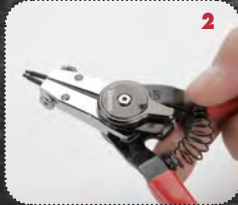
2 Knot position for external Seeger circlip® handling
