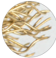
Brass Coated Steels 0,30 mm . 012"
