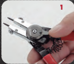
1 Knot position for internal Seeger circlip® handling
