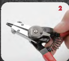
2 Knot position for external Seeger circlip® handling
