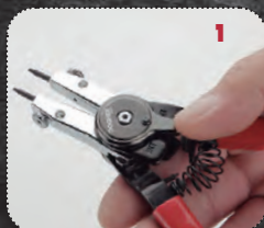
1 Knot position for internal Seeger circlip® handling
